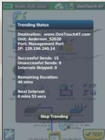
Figure 2. Trending automatically runs the AutoTest repeatedly and uploads results to the cloud
