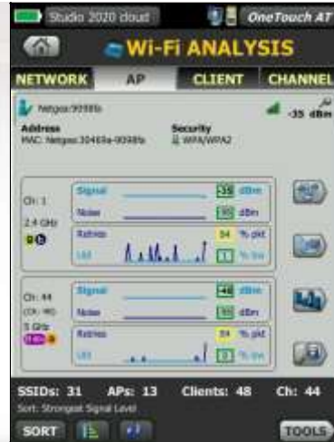
Figure 10. Visibility into Wi-Fi networks, access points, clients and channels
